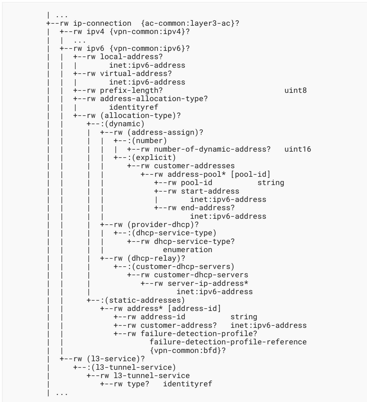
Figure 13: Layer 3 Connection Tree Structure (IPv6)
